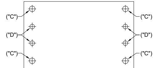
4 BASE PLATE HOLE LOCATION DIAGRAM NOTE: ISOLATOR BASE PLATE IS TO BE USED FOR HOLE LOCATION MARKING ONLY AND NOT AS A DRILLING GUIDE.
